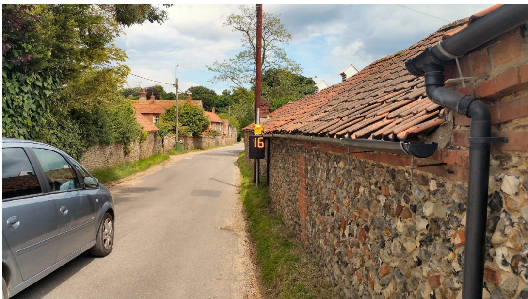
Photo of the SAM2 in action in Bridge Street. The sign flashes to the driver their speed. The computer within the sign also records the number of vehicles, the time they were recorded and their speed
